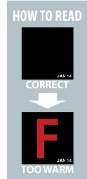
When the temperature of the refrigerator/chiller/freezer is functioning correctly, the monitor will be completely black. As the temperature of the unit increases, a number or letter will begin to be visible in the center of the monitor. The hotter the unit, the more pronounced and brightly colored the number or letter will be. When the whole number or letter in the center of the monitor is clearly visible and either red or blue in color, there is a potential temperature problem with the unit.
